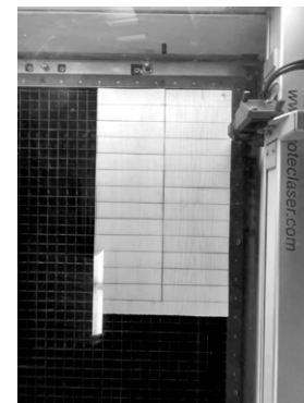
Step 3. Laser cutting veneer sheets into strips (9.5 cm x 2.2 cm x 1.4 cm)
