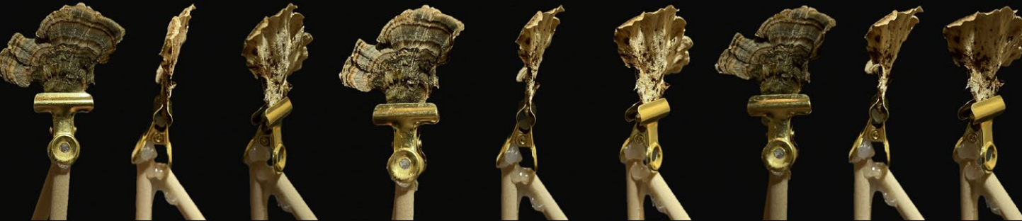
10% humidity @ 60° - 2 minutes 10% humidity @ 60° - 3 minutes 10% humidity @ 60° - 5 minutes
