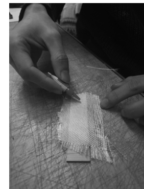
Step 4. Laminating veneer with fiberglass and cyanoacrylate to create final samples
